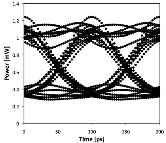
Fig. 4. Eye diagram of the recovered signal, result of the overlap of the 32 periods of the pattern.
