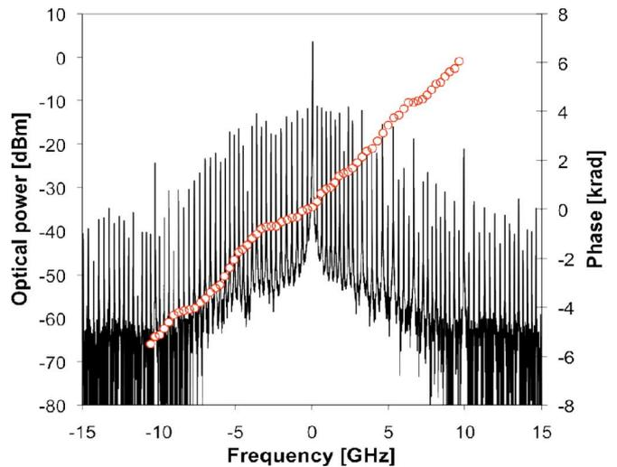
Fig. 2. Measured complex optical spectrum of a 32-bit pattern modulated at 10 Gb/s with an EAM. The solid line represents the optical power and the circles represent the accumulated phase for each spectral component. Phase reference is set to the carrier wavelength.
