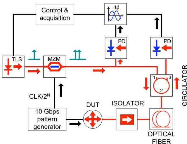
Fig. 1. Experimental setup for the measurement of the phase spectrum.
