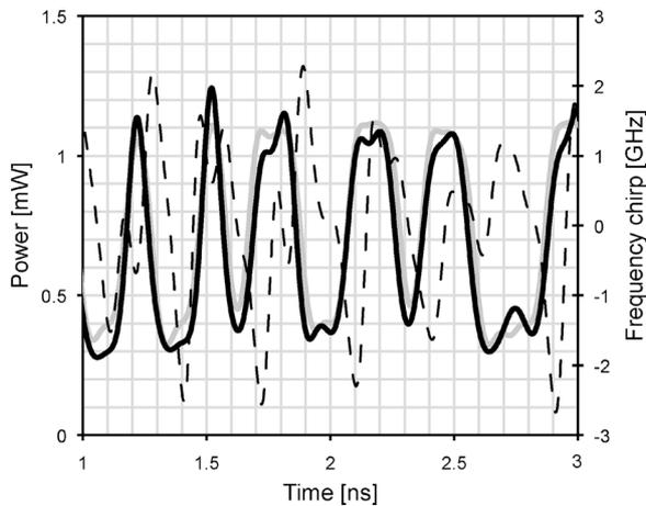
Fig. 3. Recovered instantaneous power (solid black) and frequency deviation (slashed black) from the inverse Fourier transform of the measured complex spectrum. A measurement of the modulation power by an oscilloscope (gray) is provided for comparison.
